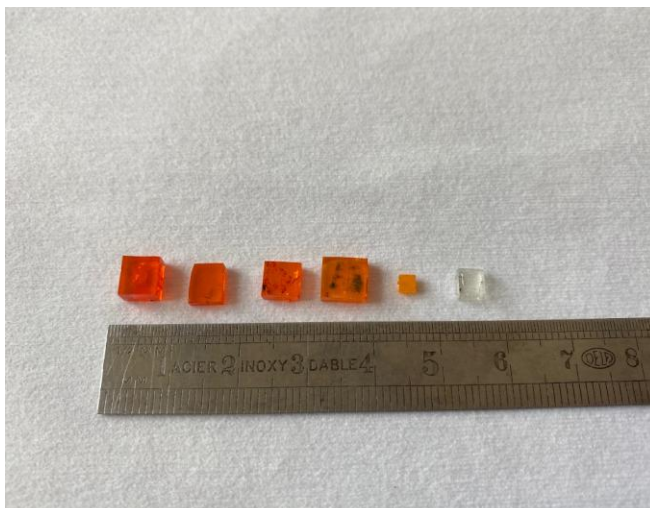
Optical image of resulting SCs: from left to right, MAPbBr 3 , MAPb(Br 0.98 Cl 0.02 ) 3 , MAPb(Br 0.97 Cl 0.03 ) 3 , MAPb(Br 0.94 Cl 0.06 ) 3 , MAPb(Br 0.89 Cl 0.11 ) 3 and MAPbCl 3
